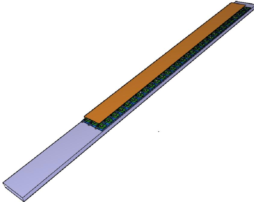
Figure 6: A SciTil super-module composed of 90 quad modules shown on top of a DIRC bar box.
