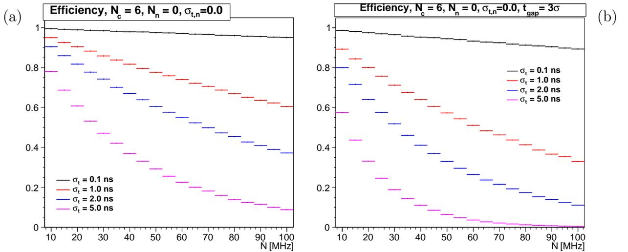
Figure 3: Event rate dependent efficiency based on pure overlap (a) and on an event building algorithm (b) described in the text for reactions with  $N_c = 6$  charged tracks. The values are plotted for instantaneous rates between 10 MHz and 100 MHz and time resolutions of  $\sigma_t \in \{0.1, 1.0, 2.0, 5.0\} \text{ ns}$ , colored in black, red, blue and magenta, respectively.
