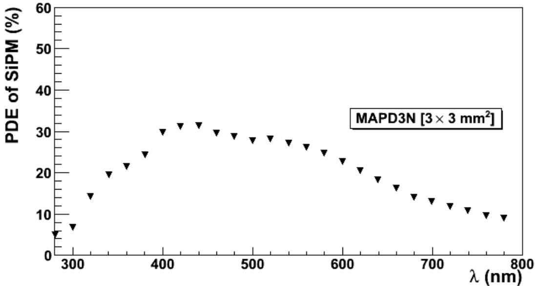
Figure 11: Photon detection efficiency of the Zecotek sensor from the MAPD3N series with 15000 pixels/mm<sup>2</sup>.
