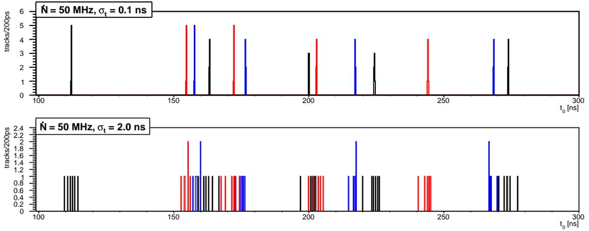
Figure 2: Illustration of  $t_{0,i}$  distribution of reactions with 6 tracks at an instantaneous rate of  $\dot{N} = 50 \text{ MHz}$  and total time resolutions of  $\sigma_{t1} = 100 \text{ ps}$  (top) and  $\sigma_{t2} = 2 \text{ ns}$  (bottom). The three color black, red, and blue are cyclically used to mark time signals  $t_{0,i}$  from different events.
