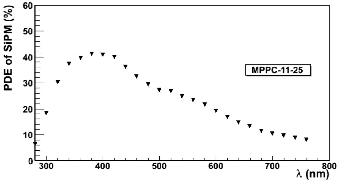
Figure 10: Photon detection efficiency of the Hamamatsu sensor from the S 10362-11 series with 400 pixels/mm<sup>2</sup>.
