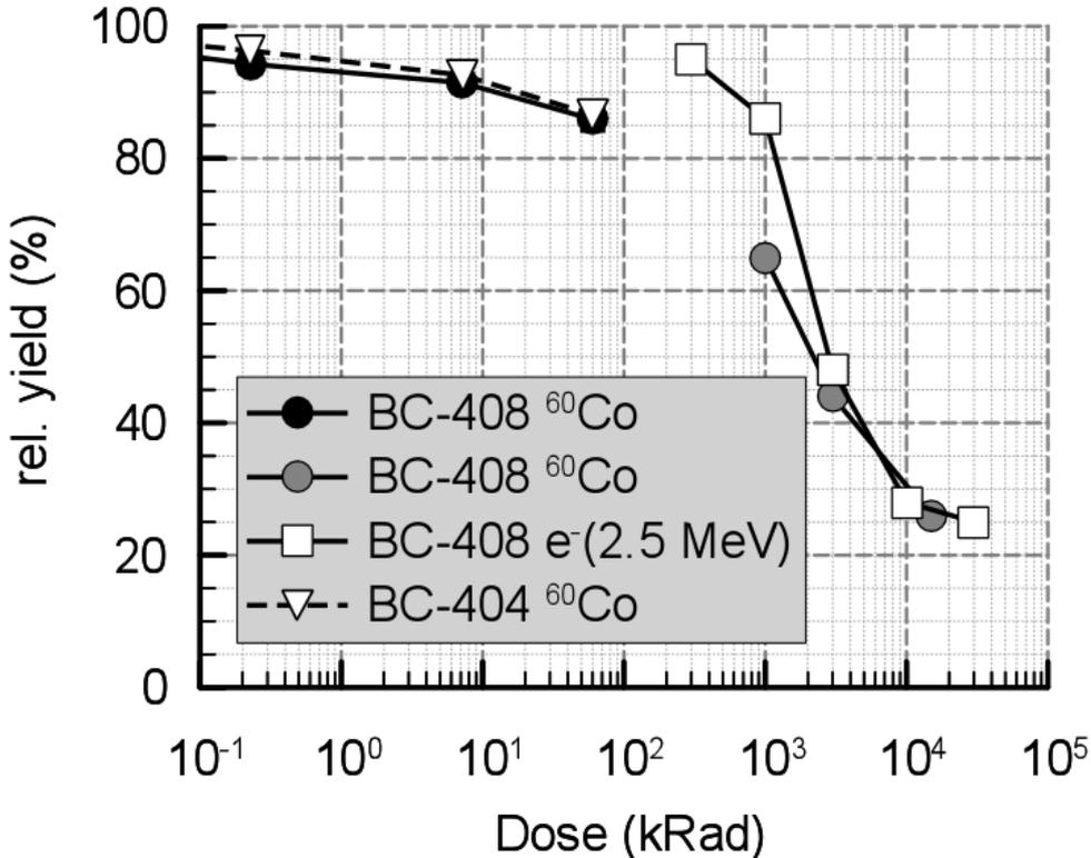
Figure 9: Relative light yield of BC-404 and BC-408 scintillators irradiated with gammas from <sup>60</sup>Co and electrons with energies of 2.5 MeV. Black circles and white triangles from [19], gray circles from [21], white squares from [20]
