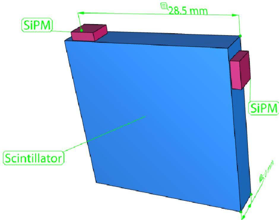
Figure 4: A single scintillator tile with SiPMs attached.
