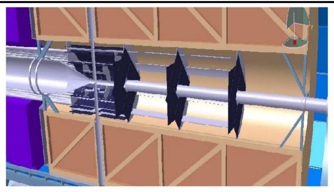
• 2 additional silicon disks at roughly Z = 800 and Z = 1100, 30mm < r < 150mm, similar to the last two MVD disks but only silicon strips (so far)
