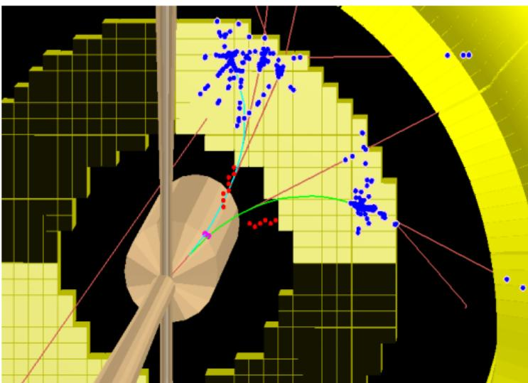
Red lines corresponds to photons track, blue line - electrons track and green line - positron. Pink points are hits in MVD, red pointat are hits in STT and blue points are EMC hits.
