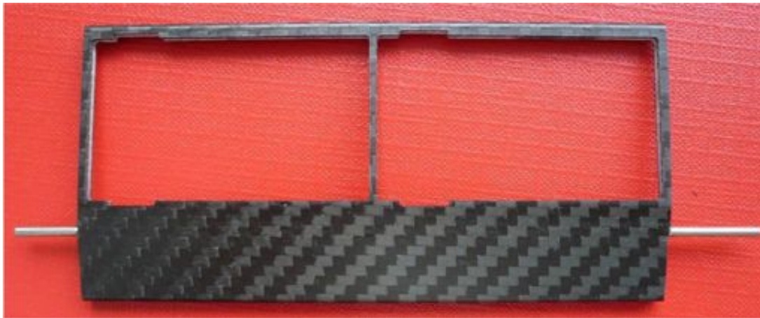
Reduced size stave with carbon foam and pipe
