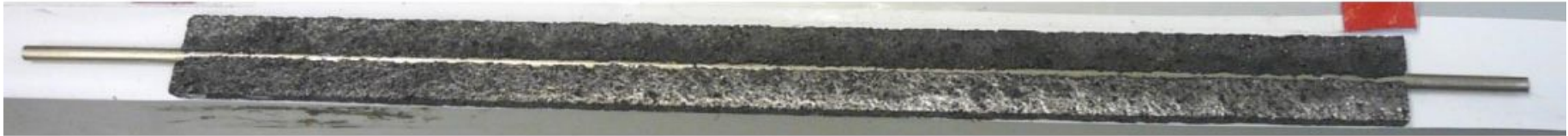
Cooling pipe embedded in the carbon foam
