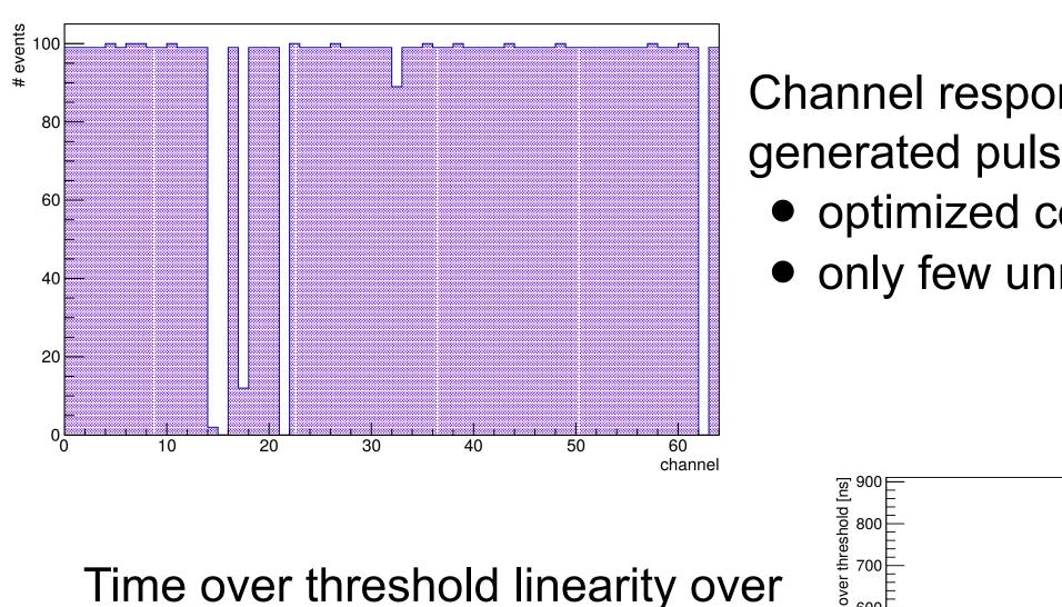
Channel response for 100 internally generated pulses of 20 fC charge each:
