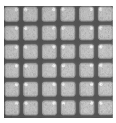
Bond pad distribution reflects the double column structure of the readout chip.
