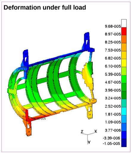
Two halves clamped around the beam/target pipe.
