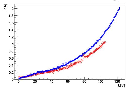
All irradiated capacitors show a higher leakage current than their non-irradiated equals, but only at voltages above their rated voltage. 0603 - capacitors
