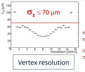
Primary and secondary vertex resolution:  $\sigma_{x,v} \leq 35~\mu\text{m}~/~\sigma_z \leq 100~\mu\text{m}$
