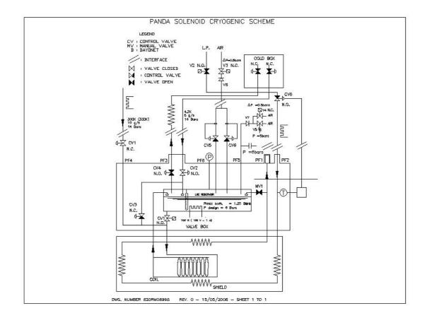
Figure2, Flow diagram of Natural Convection refrigeration system
