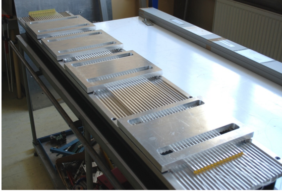
Figure 5.21: Prototype module mounted on the transfer frame (left) and the way of transferring (right).
