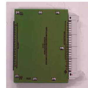
Discrete preamp from Krakow used during straw tests
