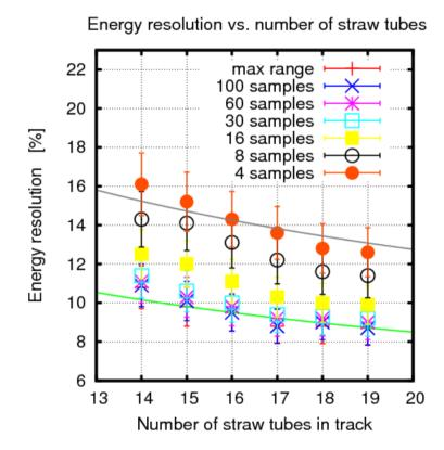
Since almost whole charge is comprised in the first 40 – 60 samples shortening of the integration up to 30 samples causes only minimal deterioration of the energy resolution.
