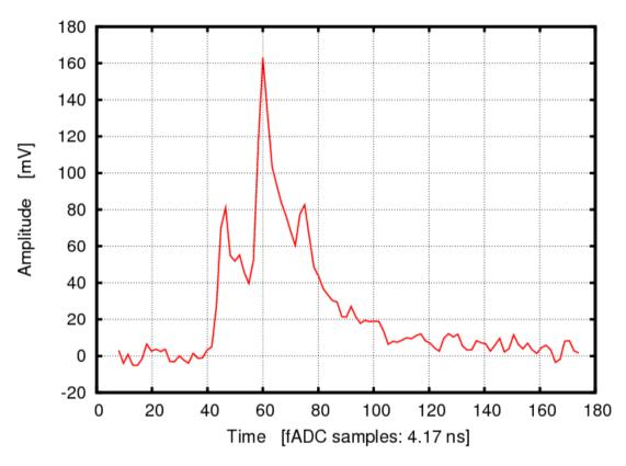
Response of detector and electronic is proportional to the primary ionization
