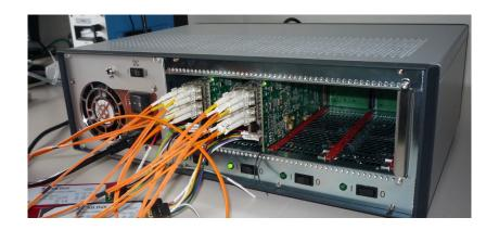
• Tested one xFP channel of two card in a MicroTCA with 6.25 Gbps; without errors.
