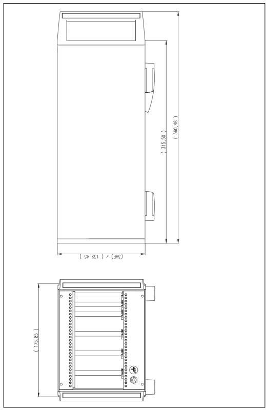
Figure 11: Mechanical Dimensions 21850-045/-081
