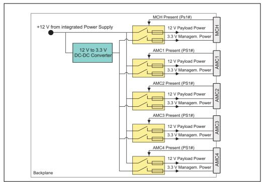
Figure 7: Power Distribution (Without Power Management Board)
