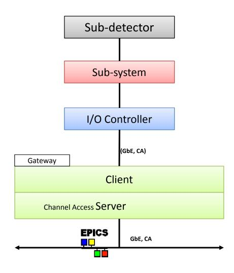
**I/O Controller (IOC)**: Any device (PC, SBC, COM, micro-controller board, FPGA board etc.) able to manage the I/O of the sub-system;
