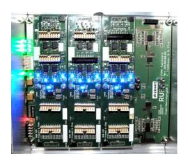
THMP: Temperature and Humidity Monitoring Board for PANDA
