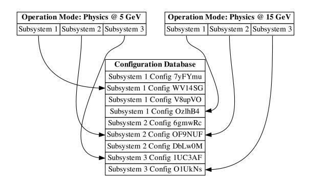
Figure 2: Block diagram showing the assignment of configuration datasets to operation modes.
