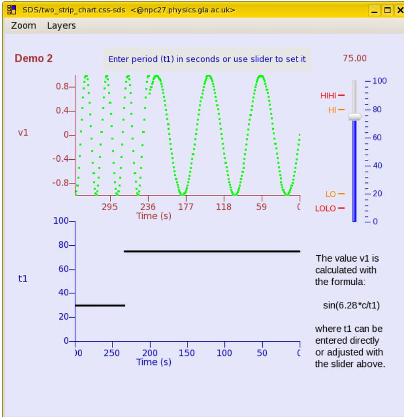
A more complicated example to demonstrate the possible use of CSS in the PANDA collaboration was also created. This GUI could be used to control a dipole magnet which will be part of the hardware used in the PANDA collaboration. This example included warnings (in the form of a colour change) if the EPICS variables exceeded a certain range set in the EPICS database. A screenshot of this GUI is shown below
