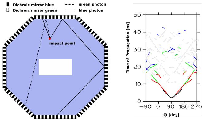
Fig. 4. Sketch of the lightpath in the ToP Disc. The pattern on the right side is spreaded by the numbers of reflections the photons underwent.
