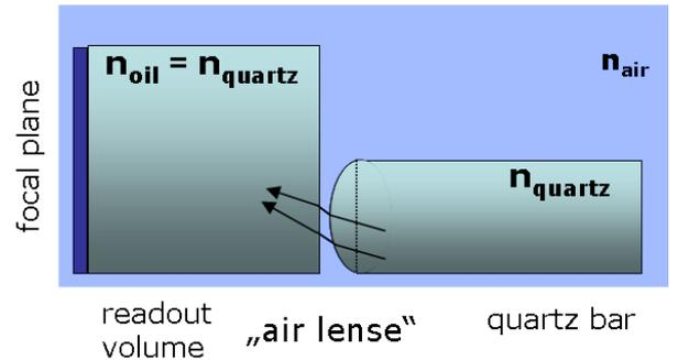
Fig. 3. Sketch of a photon readout with an air lens.
