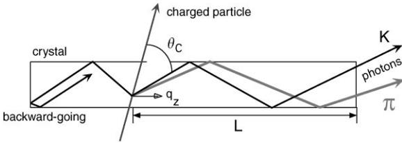
Fig. 1. Side view of propagating photons. TOP is inversely proportional to  $z$ -component  $q_z$  of the light velocity:  $\text{TOP} = (L \times n(\lambda))/c q_z = 4.90 \text{ ns} \times L \text{ m}/q_z$ .  $\theta_C$  is the Cherenkov angle and  $L$  is the particle injection position from the bar-end. At the opposite end, a mirror is placed to reflect the BW photons.
