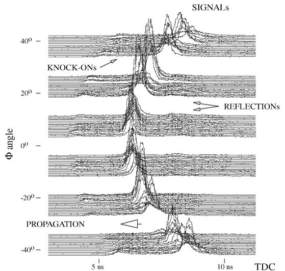
Fig. 7. Cherenkov ring image measured by TOP counter for normal incident 4 GeV/c  $\pi^-$ s at  $L = 1$  m.
