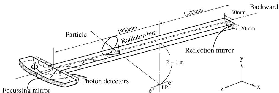
Fig. 2. Structure of the TOP counter. Basic parameters are indicated in the figure. Since KEKB is an asymmetric collider, the quartz bar is accordingly configured  $z$ -asymmetric relative to the interaction point (IP).
