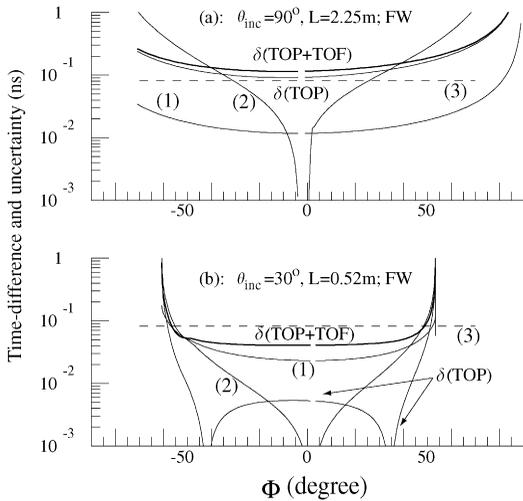
Fig. 3. TOP difference and three dominant contributions for 4 GeV/c K and  $\pi$ . The counter is supposed to be configured at KEKB-BELLE under  $B = 1.5$  TG, as shown in Fig. 2, and only FW photons are detected.  $\delta(\text{TOP})$  and  $\delta(\text{TOP} + \text{TOF})$  are the difference of respective times between K and  $\pi$ , and (1), (2) and (3) are the smearing contributions described in the text.
