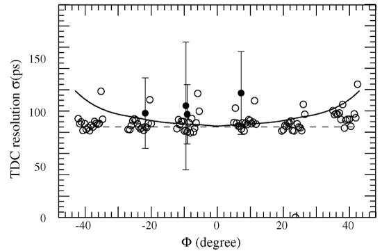
Fig. 6. Measured time resolutions for normal incident 2 GeV/c  $\pi^-$ s. Open circles are obtained at  $L = 0.02$  m. The closed circles are obtained at  $L = 1$  m as described in the text and the curve is the expected one based on the measurement of  $L = 0.02$  m.
