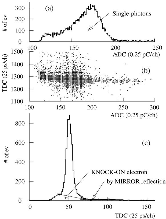
Fig. 5. ADC and TDC distributions of 20th channel for the normal incident 2 GeV/c  $\pi^-$ s with  $L = 0.02$  m. Timewalk correction was applied in (c) and the time resolution of trigger uncertainty subtracted is  $\sigma = 80$  ps.
