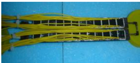
Figure 5.37: Prototype of two staves of the second layer of the barrel, with dummy chips (resistors), with a power of about 21 W for each staff.
